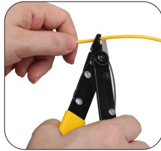
2. Remove cable jacket 50mm.
