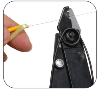
4. Strip off 250um coating 23mm, in two times to avoid fiber damage.
