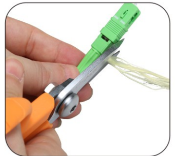
12. Trim the excess Kevlar with the Kevlar scissors.
