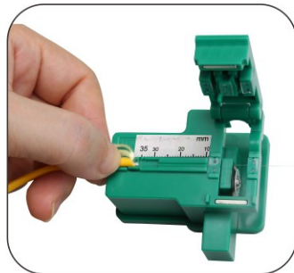
6. Set fiber on the cleaver at 35mm cleave-length. Cleave the fiber.
